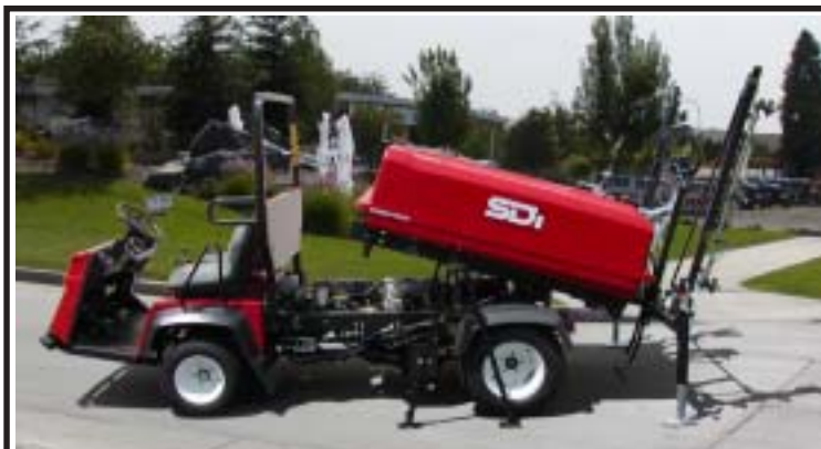
Optional EZ on/off mounting using the "Quick Stand" Sprayer Storage Stand.
