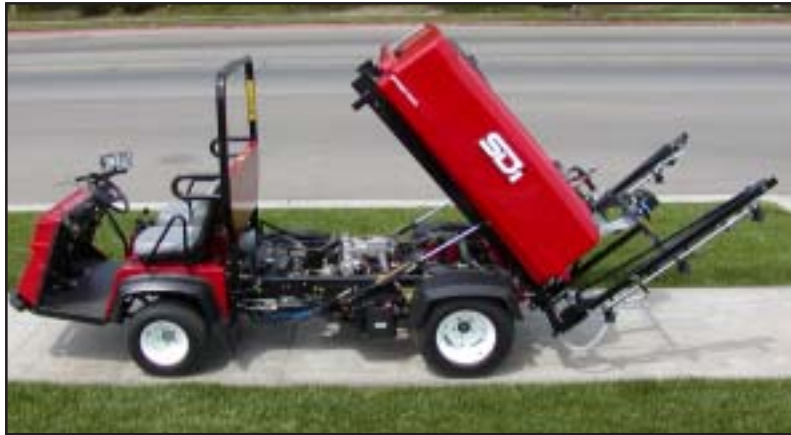
Sprayer raised for accessibility to engine.
