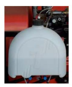
The compact air compressor and control valves are located behind the 4 quart liquid solution tank with solution metering valve.
