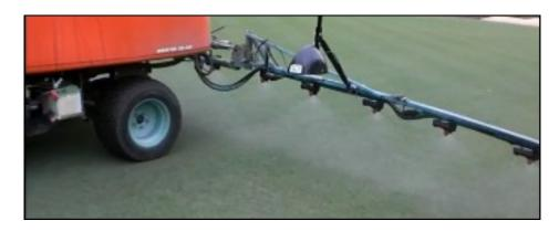
When the distance between the spray boom and the ground changes, the consistency of your spray application changes. A boom wing that is too close to the ground can cause streaking, if it is too high you can dilute the rate. Either way it can change the efficacy of any pesticide or nutrient you apply. In days past you just had to accept an uneven application, now you can take control of this variable in your spray application!
