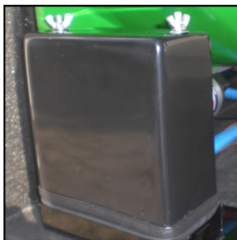
Separate battery to power the pumps is recharged by the vehicle.
