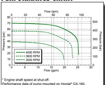
Performance data of pump mounted on Honda® GX-160.
