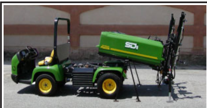
Optional EZ on/off mounting using “Quick Stand” Sprayer Storage System.
