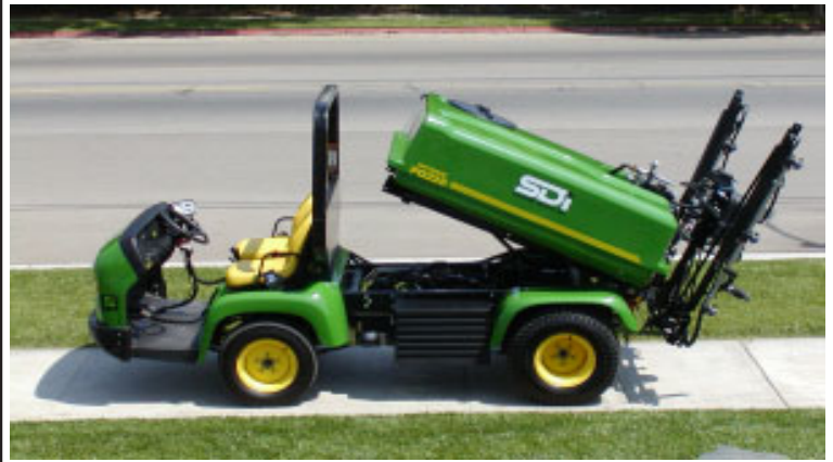
EZ access to engine area using hydraulic lift cylinder.
