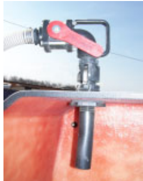
Above: Fill nozzle in bypass position (filling & circulating).
