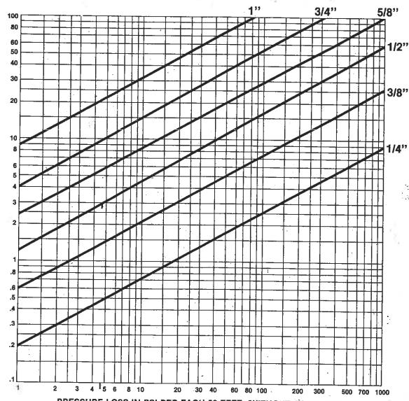
PRESSURE LOSS IN PSI PER EACH 50 FEET, (WITHOUT COUPLINGS)
