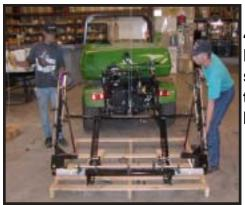
4. Raise the boom up slowly until the approved safe lifting device has the boom suspended above the shipping skid (use caution while raising the boom to the hanging position to avoid damaging the nozzle bodies on the center boom section)
