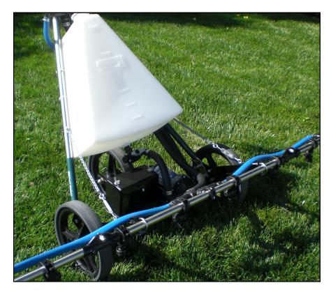
The **Turf Walker SC6** from SDI features a spray tank, stable tricycle chassis, 12 volt pump with rechargeable battery and a folding 6.5 foot (2 meters) wide spray boom with 8 drip free nozzles.
