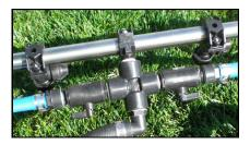
The folding boom is constructed from stainless steel tubing. The 8 nozzle bodies with diaphragm check valves are connected directly to the boom. Using the ball valves shown above, you can direct flow to either or both wing sections. The center section is always active during spray operations.
