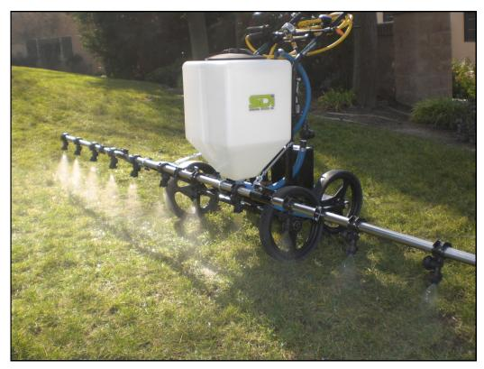
The **Turf Walker SC10** from SDI features a 10 gallon spray tank, 12 volt pump with rechargeable battery and a folding 10 foot (3 meters) wide spray boom with 12 drip free nozzles on 10 inch centers. Each boom section can be individually controlled.
