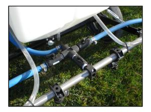
The folding spray boom is constructed from stainless steel tubing and has 12 nozzles with diaphragm check valves. Each boom section can be controlled separately.
