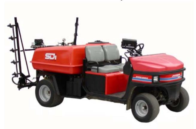
*Model Shown:* VM225D/DS equipped with the OTB15/10-3 triple nozzle Greens & Tees Boom and the Raven SCS440 Spray Controller fitted with SDI's Motorized Boom Valves.
