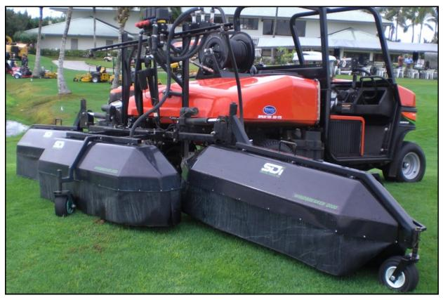
Do windy days put a hold on your spray operations? The SDI Windbreaker 2000 Shielded Spray Boom offers you the ability to spray at those times you are unable to use a conventional spray boom because of wind or potential drift problems. The 15 foot wide spray boom has three individual floating sections that maintain a consistent spray height over undulating terrain.
