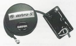
**WIRING:** Route the 10 foot cable from the receiver into the cab (if receiver is externally mounted). Avoid sharp edges or heat sources. The rectangular module is roughly the same size as the connector and will fit through the same opening.
