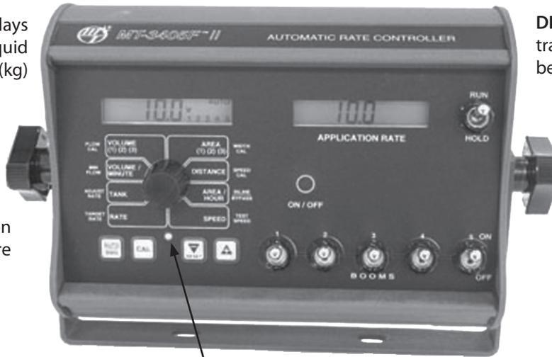
**DISTANCE:** Displays distance traveled in feet (meters). May be reset.
