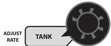
**Auto Delay Time:** Typically used when using relatively slow ball valves for boom shut-off, this feature delays adjustment of the servo valve until the boom valves are open. Use “+” and “-” buttons to set from zero (OFF) to 4 seconds.
