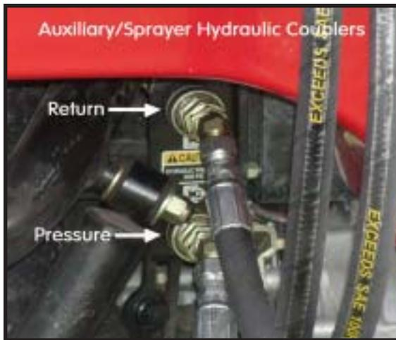
1. Locate and identify the two hydraulic hoses at the rear of the sprayer and attached to the spray pump's drive motor (one marked pressure the other marked bypass/return)
