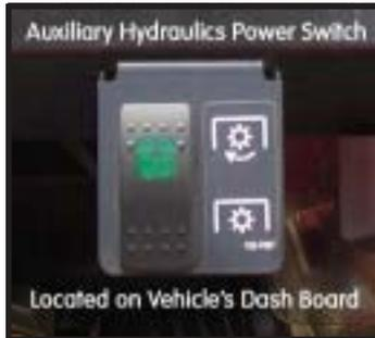
4. Locate the auxiliary hydraulics on/off switch on the vehicle's dash (two possible locations: to the left of the steering wheel or below and left of the speedometer)
