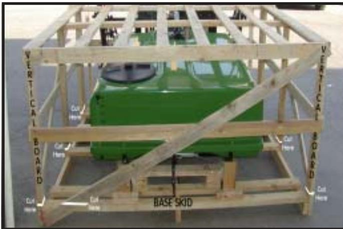
1. Use a reciprocating saw to cut the vertical support boards just above the base of the skid (do not hit the sprayer with the blade)
