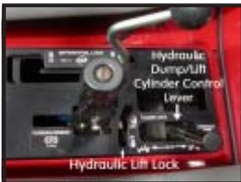
11. Once installed, you will be able to use the Workman's® hydraulic dump/lift cylinder control lever to raise and lower the sprayer for access to the engine compartment for service operations (remember to always use the "Bed Safety Support" while sprayer is raised)
